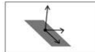
Accelerometer Logs acceleration in 3 dimensions relative to gravity
